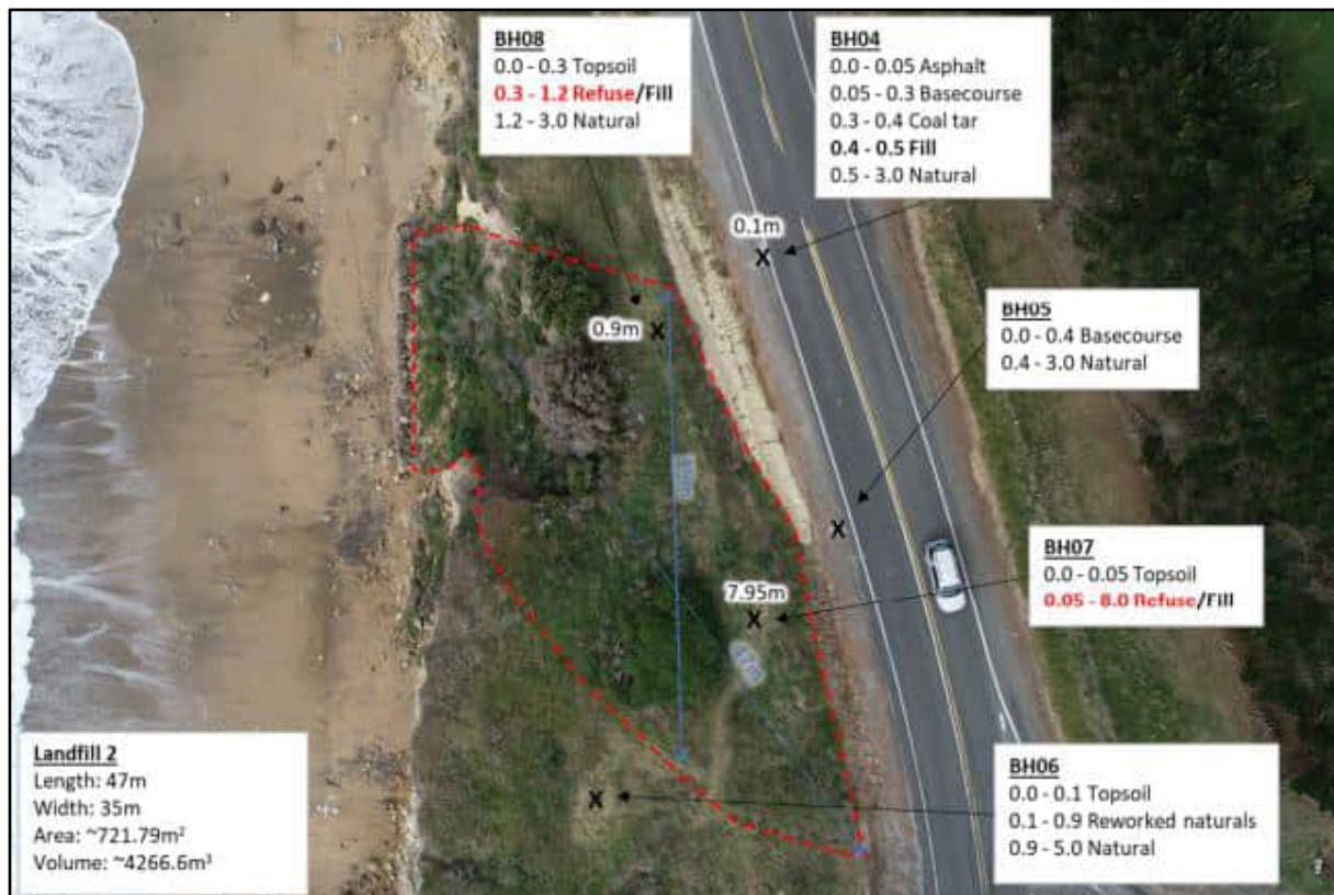
Figure 6 Location of WSP (2021) borehole investigations at Landfill 2 (extracted from WSP 2021 report).
