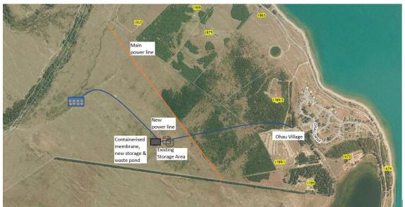
Figure 2.1: Schematic of Proposed Option 3
