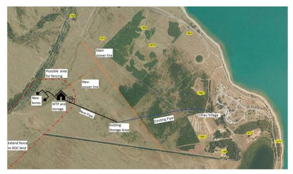
Figure 2.3: Schematic of proposed option 5
