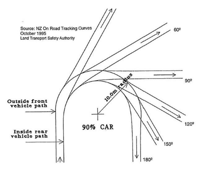
Note: Minimum recommended clearance for both sides of the vehicle 600mm.
