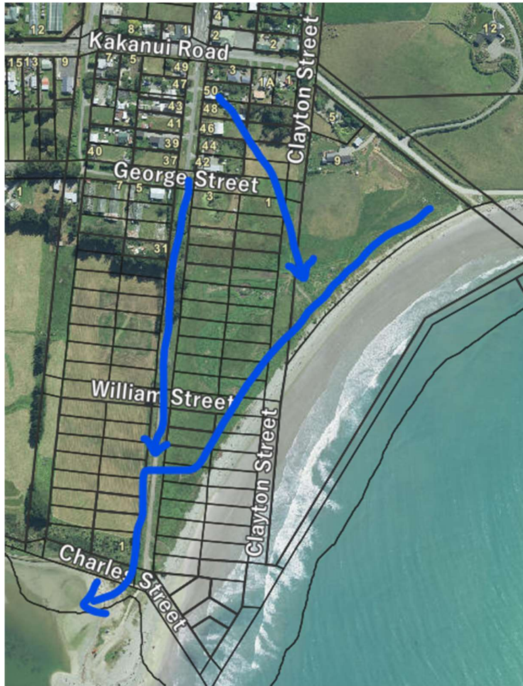
Figure 7: Aerial photo and annotation showing the existing important drainage network that assists in directing both stormwater and coastal inundation water away from properties and assets in the subject area.
