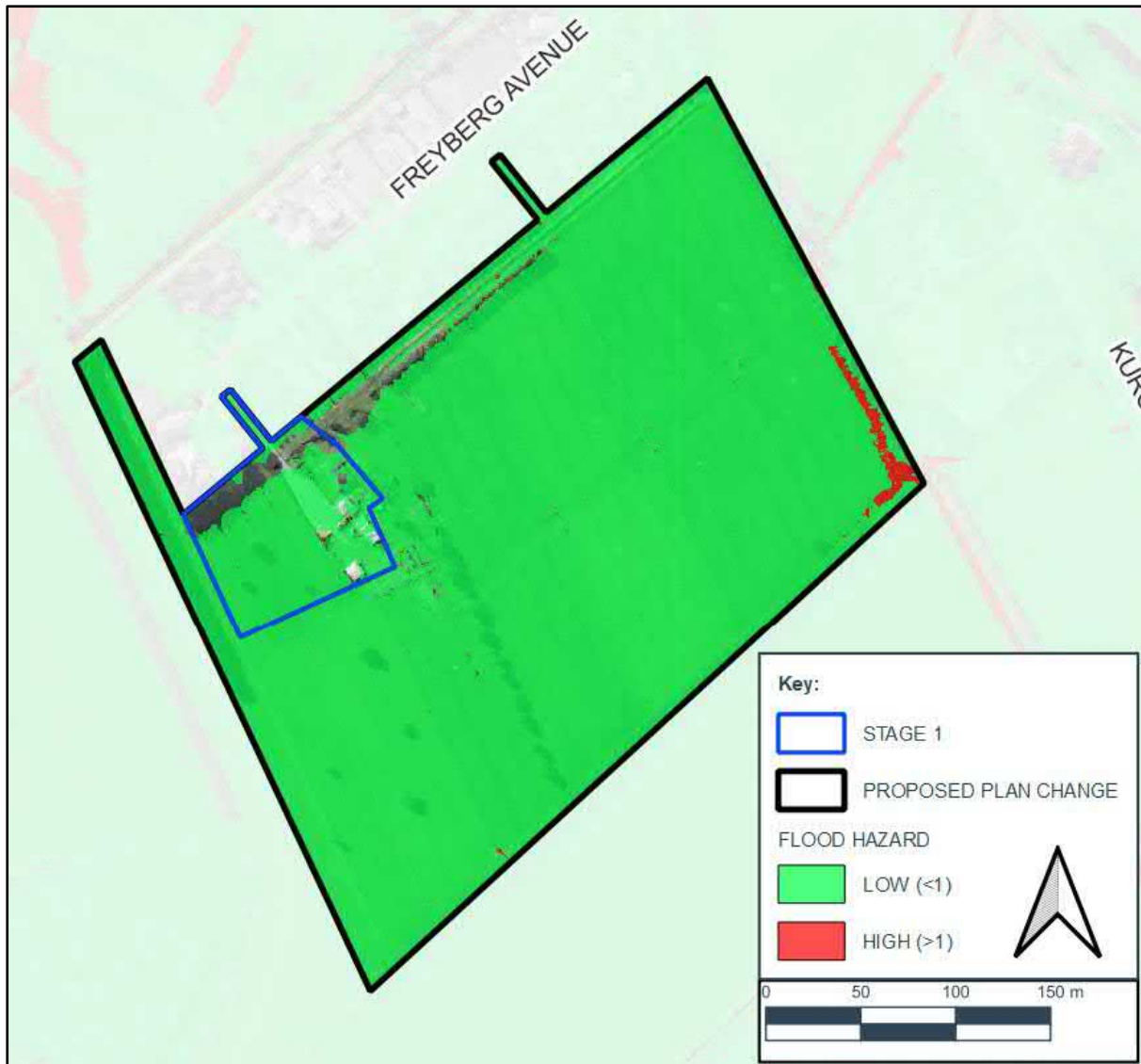
Figure 2: Predicted flood hazard for the 0.2% AEP Event
