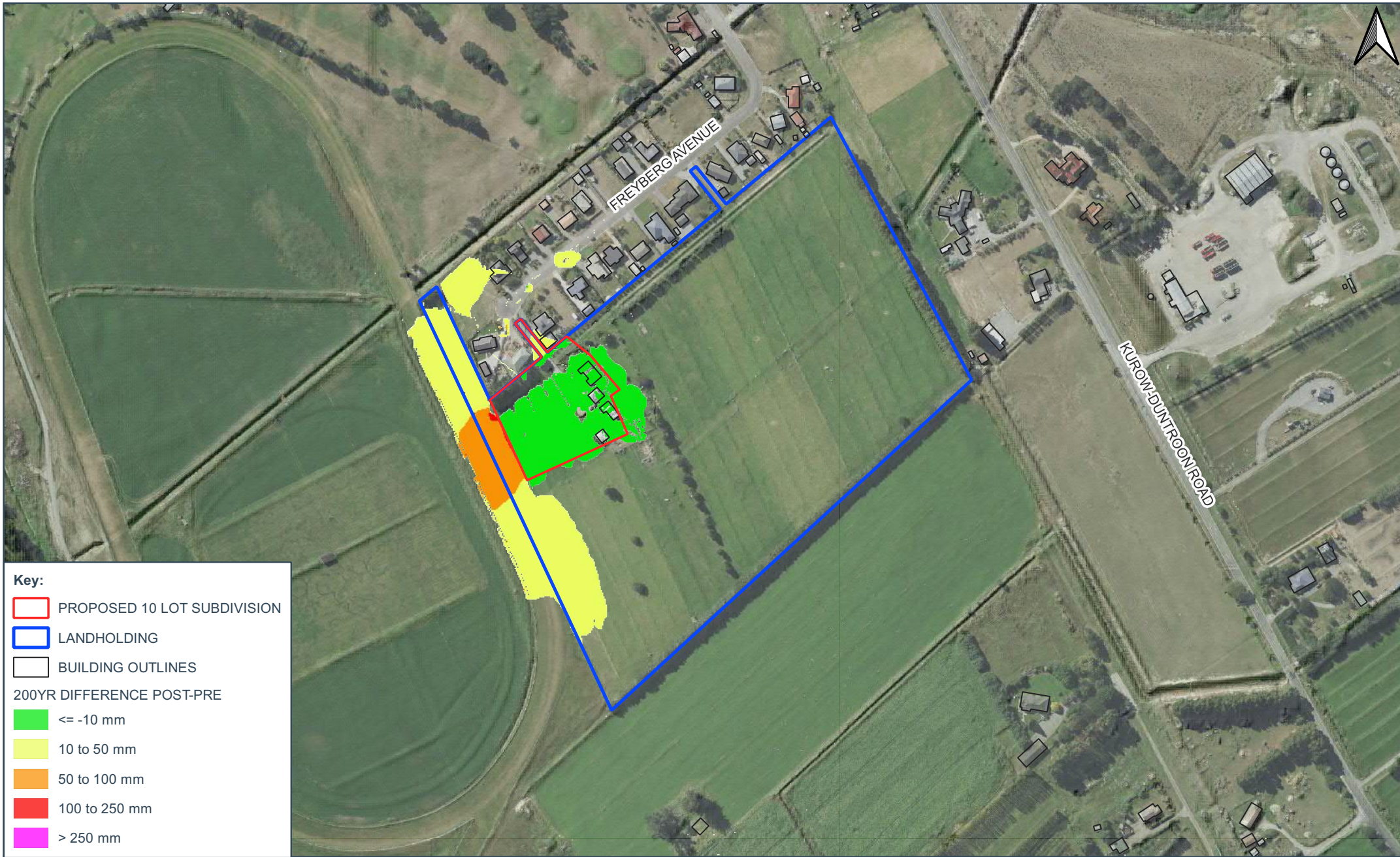
FIGURE 6: DIFFERENCE IN FLOOD ELEVATION FOR THE 200YR EVENT (POST - PRE). NOTE, DIFFERENCES LESS THAN 10MM NOT SHOWN 20 of 23 SOURCE: LINZ basemaps Maps made with QGIS
