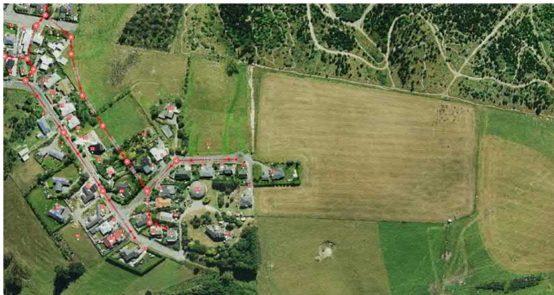
Figure 12: Aerial image from WDC GIS Maps showing the nearby sewer reticulation.
