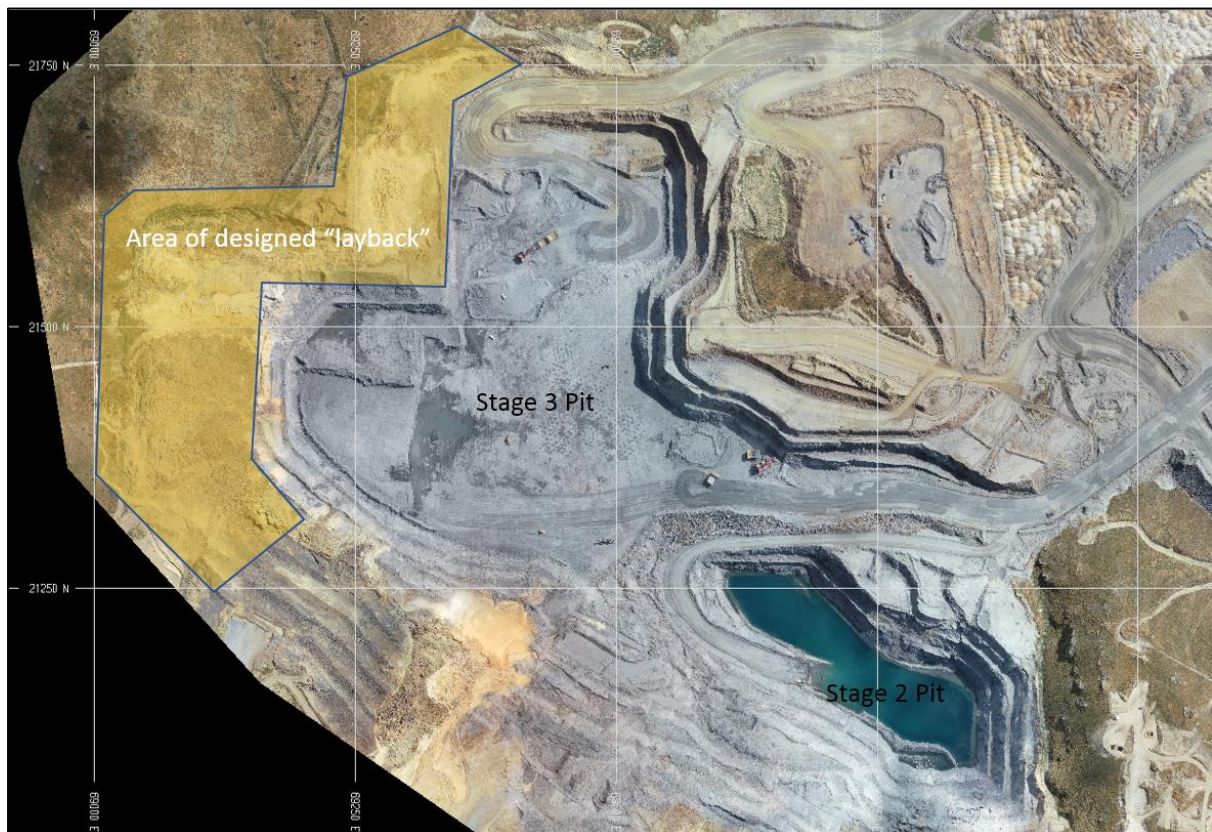
Figure 1. Aerial view of the Coronation North pit showing the area required to be laid back.
